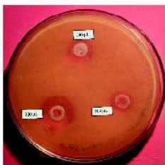
Fig. 3 Inhibition zones for different amount of ZnO nanopowders calcined at 400 °C
